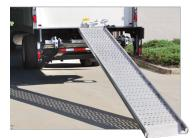
Optional walk remp can be operated without moving the liftgate.
