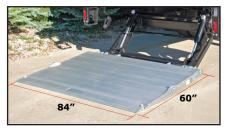
60" deep x 84" wide aluminum platform with individually replaceable extrusion provides a large work area for handling pallet loads.
